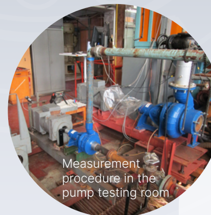
Prototype impellers including pump itself
