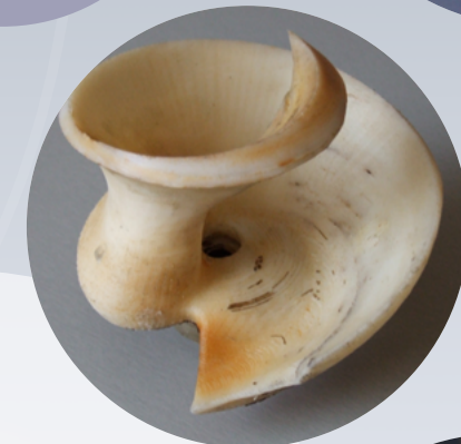
Balanced impeller (3D printout)
