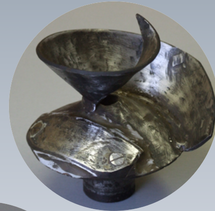
Unbalanced impeller (weldment)
